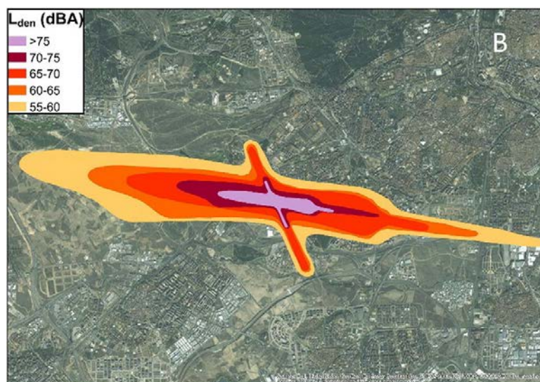
Figure 3.1 Example of noise exposure contour map (Gasco, Asensio, & de Arcas, 2017).
