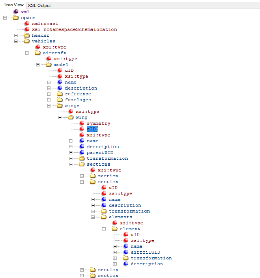
Figure 4.2: CPACS Hierarchical tree relative to the definition of the wing geometry.
