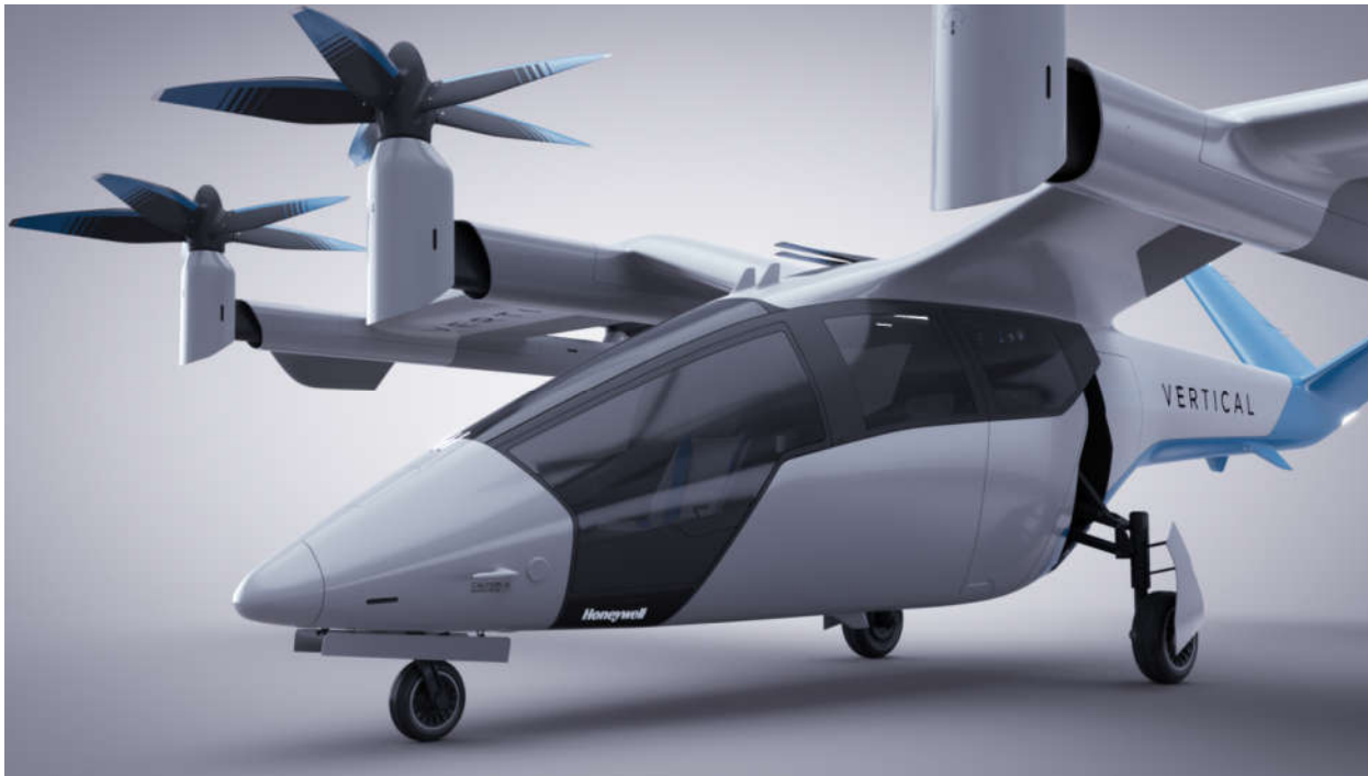
Figure 91: "Side stowing" main landing gear configuration on a novel VTOL aircraft design with limited space in the fuselage
