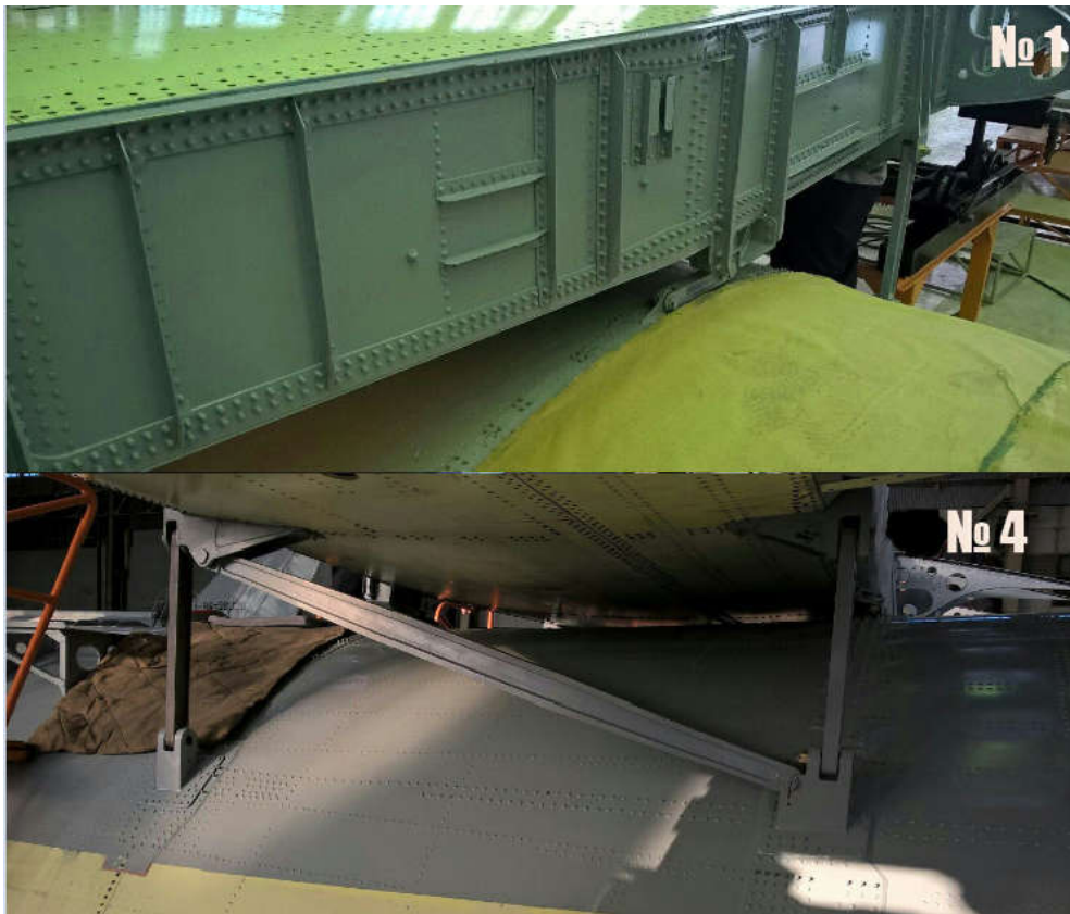
Figure 87: Fuselage wing attachment of military transport aircraft
